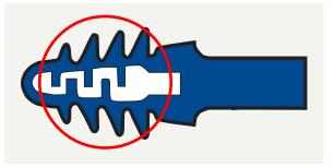
AirSoft elevates its groundbreaking air pocket design to the next level for superior protection. Utilizing advances in acoustical engineering, AirSoft's new internal fins create an interlocking, noise-blocking barrier within the air pocket, providing dependable attenuation for all wearers upon proper insertion. AirSoft also attenuates better across all frequencies, offering the highest multipleuse protection with an NRR 27.
